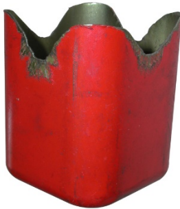
Square Deep Drawing Cup Test
