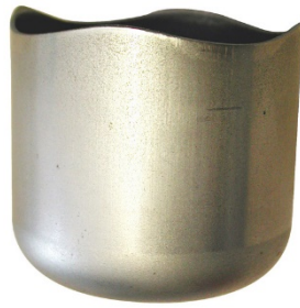
Deep Drawing Cup Test
